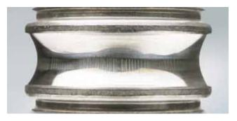
When electric current passes through a bearing, arcing and burning occurs through the thin oil film at points of contact between the race and rolling elements. The points of contact are melted locally to form "fluting" or groovelike corrugations which are seen by the naked eye. The magnification of these grooves will reveal crater-like depressions which indicate melting by arcing.
